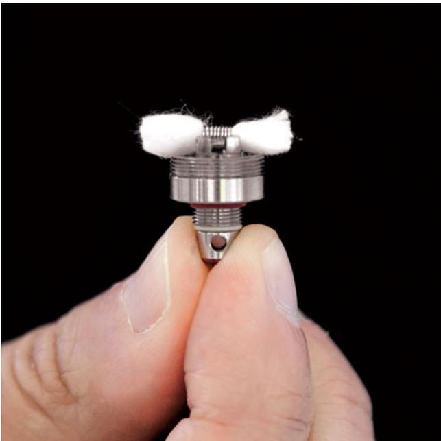
**Step 5:** Insert the cotton into the RBA base on both sides, by using a screwdriver.
